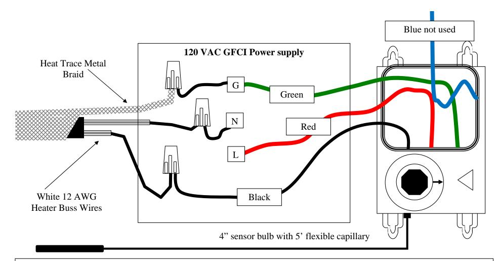
Arctic Trace Submersible Heat Trace System and TRF115 Thermostat Junction Box wiring detail
