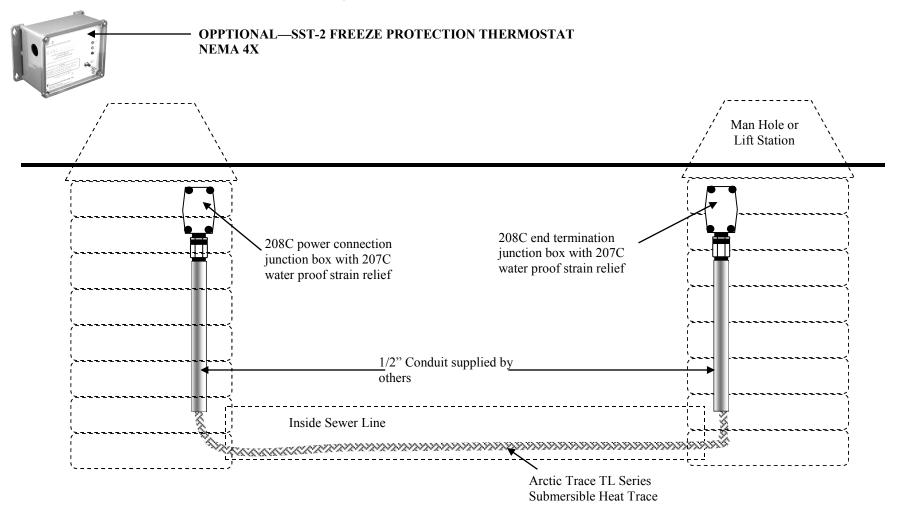
Submersible heat trace will enter water or wastewater system using a 208C junction box. Heat cable will run inside the piping system to protect any unconditioned area from freezing.
