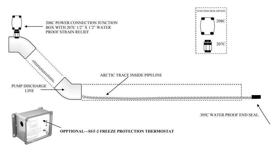
Submersible heat trace will enter the piping system using a 208C or 206C ½" MNPT connection. Heat cable will run inside the piping system to protect any unconditioned area from freezing.
