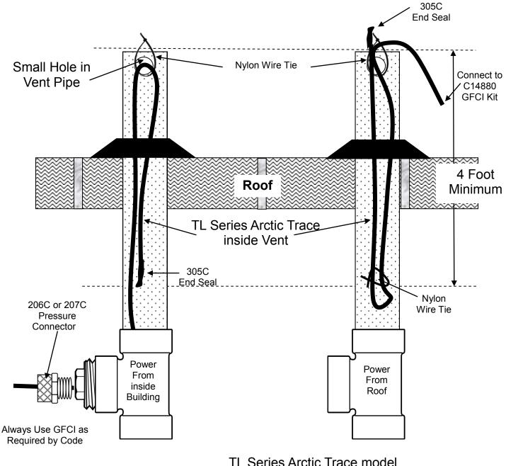
TL Series Arctic Trace model Z121012CBTL, 10 watt per foot at 120Vac.
