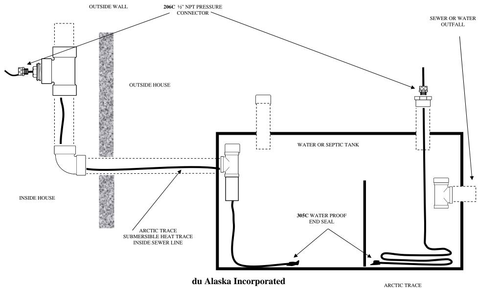
6706 Greenwood Street, Anchorage, Alaska 99518 Phone (907)-522-3004 Fax (907)349-1023 ARCTIC TRACE SUBMERSIBLE HEAT TRACE LOOSELY COILED IN TANK
