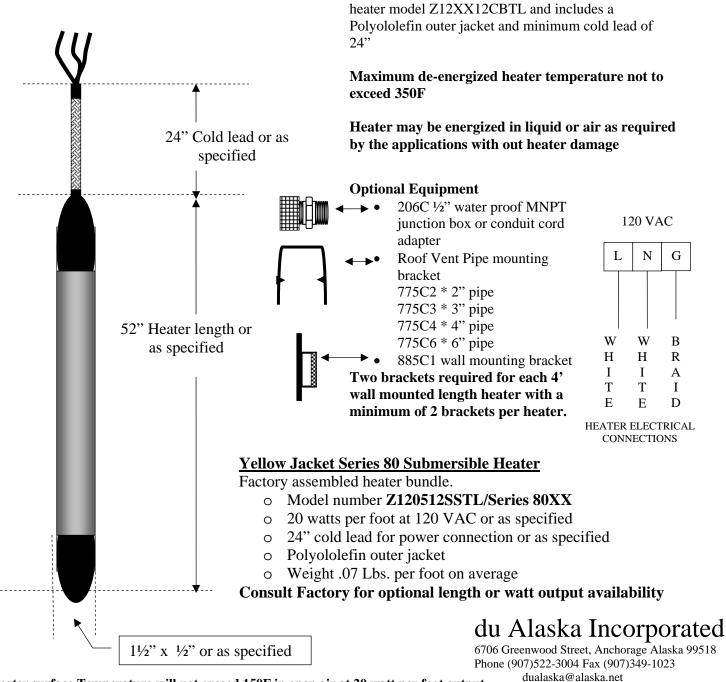
Heater surface Temperature will not exceed 150F in open air at 20 watt per foot output.
